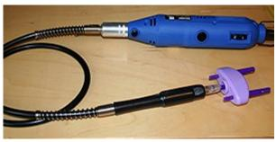
A 2 pin hair braider modified and attached to a Dremel like tool. The one pictured is a variable speed engraving multi tool with grip extension that makes leader tensioning a dream.
